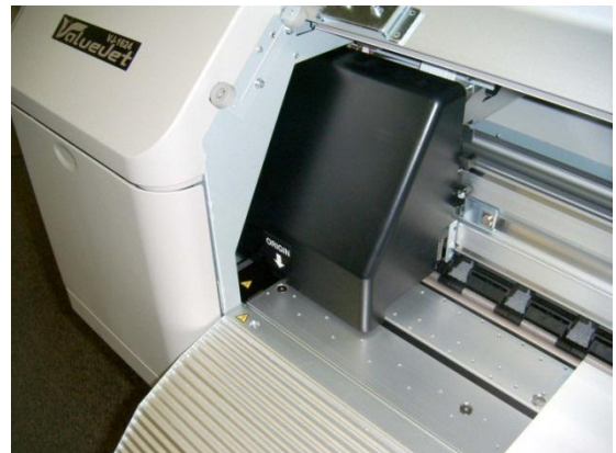
The head will move to the left maintenance station; open the maintenance cover.
