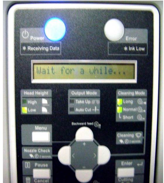
You will see the message "Wait for a while" several times during the measurement process. Do not touch anything while this message is displayed, simply wait for the next prompt.
