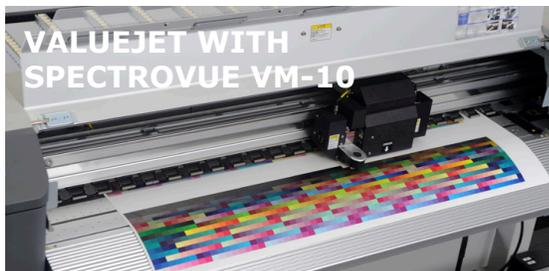
**TEST:** Mutoh ColorVerify is a new feature found on the ValueJet VJ-1324, 1624 and 1608HS large format inkjet printers. These printers all feature support for Mutoh's SpectroVue VM-10. This instrument attaches directly to the print head of the printer and is used to build color profiles, linearization files and implement in-shop process control.
