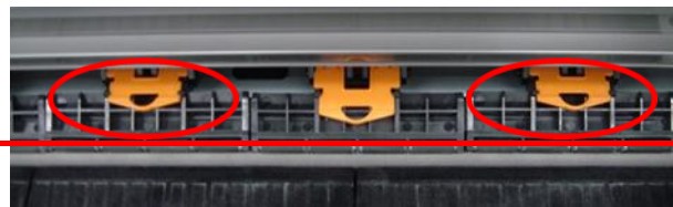
“Roller Cancel Function: ON” red encircled roller is disabled when you push orange lever
