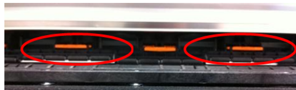
“Roller Cancel Function: ON” red encircled roller is disabled (up)
